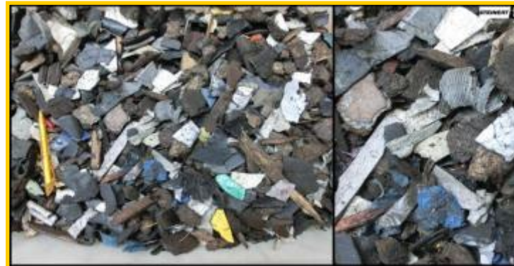
ASR light fraction after swim/sink conglomerate of plastic and wood
